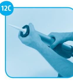
Replace front cap and ensure a tight fit to barrel.
