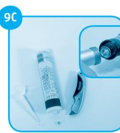
Remove cartridge and nozzle ends with a sharp knife.
